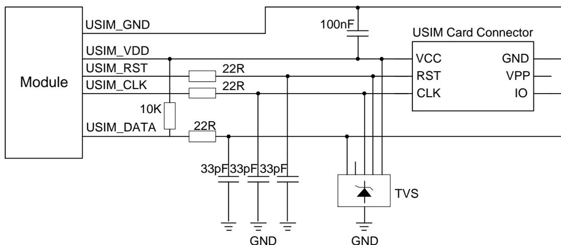
**Figure 13: Reference Circuit of USIM Interface with 6-pin USIM Card Connector**
