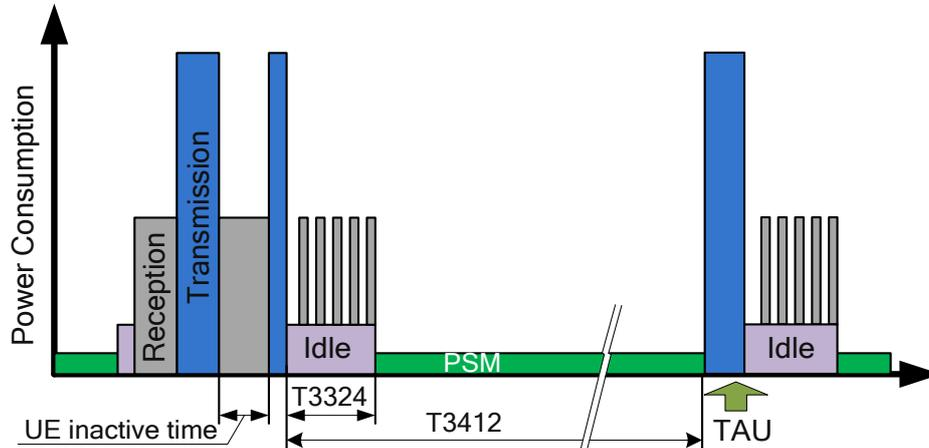
**Figure 3: Module Power Consumption in Different Modes**
