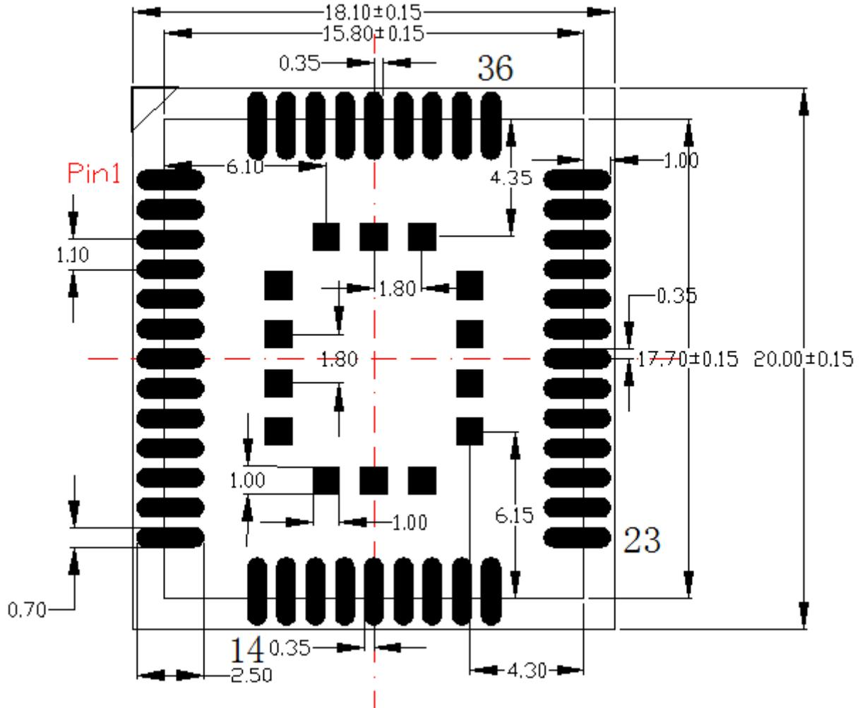
Figure 26: Recommended Footprint (Top View)
