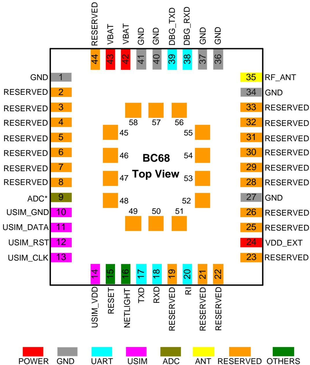
Figure 2: Pin Assignment
