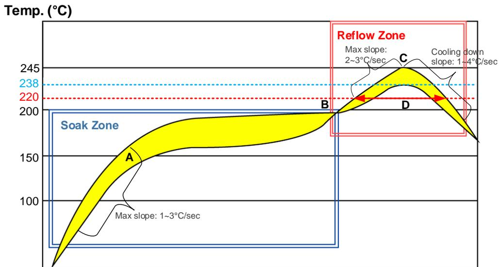
**Figure 29: Reflow Soldering Thermal Profile**
