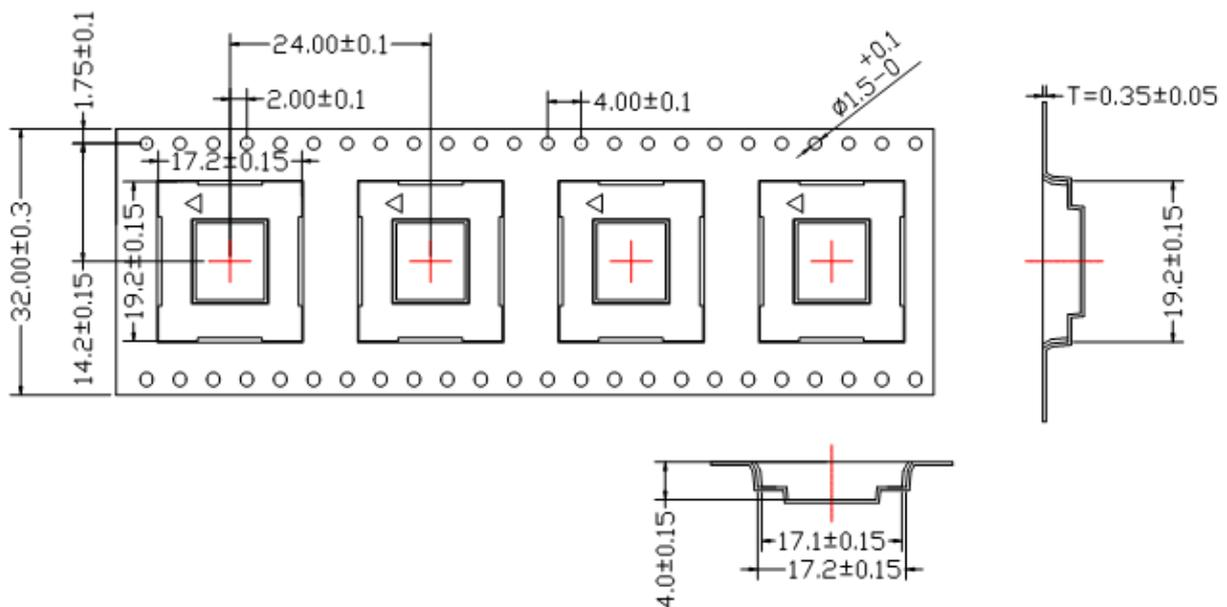
Figure 30: Tape Dimensions (Unit)
