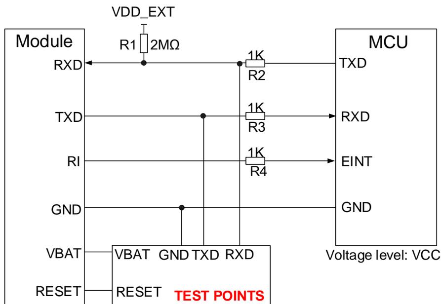
Figure 11: Level Match Design for VCC System
