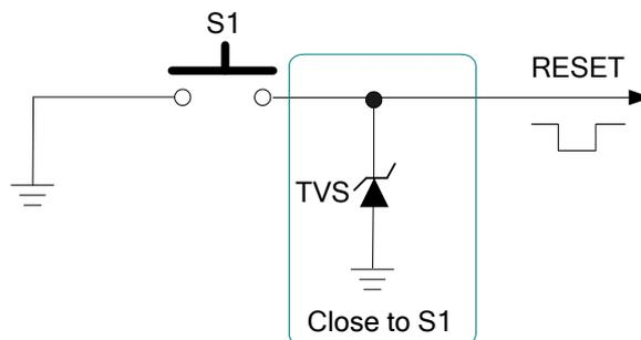
**Figure 8: Reference Circuit of RESET with Buttons**
