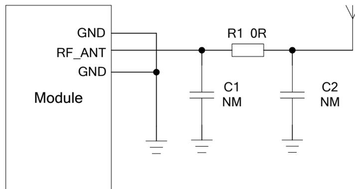
**Figure 16: Reference Design of RF Antenna**
