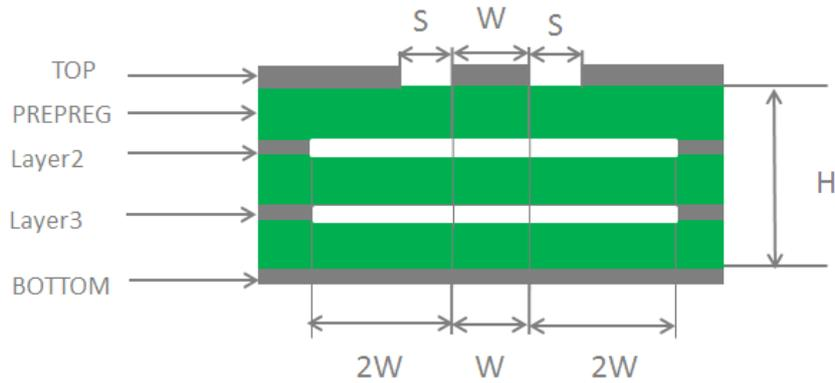
**Figure 20: Coplanar Waveguide Design on a 4-layer PCB (Layer 4 as Reference Ground)**
