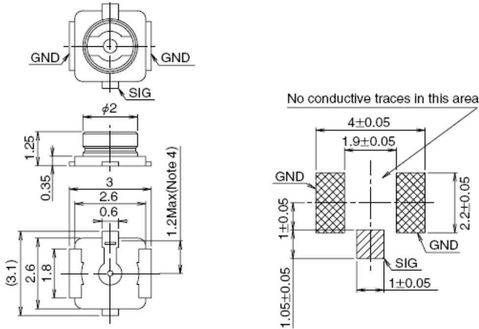
Figure 21: Dimensions of the U.FL-R-SMT Connector (Unit: mm)
