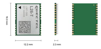
The L26-T GNSS module features high precision timing in demanding applications world-wide. The module can concurrently connect to GPS, Galileo, GLONASS, BeiDou and QZSS constellations, and use DGPS and SBAS systems for better accuracy and performance. The L26-T module also supports the outputting of multi-GNSS raw data. The module is designed and manufactured according to IATF 16949: 2016 standard.
