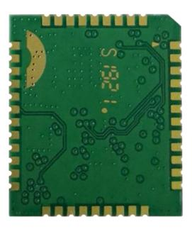
Figure 39: Bottom View of the Module
