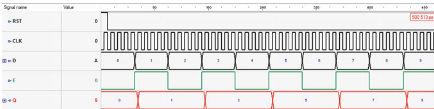
Fig. 2.22 Simulation parallel-parallel enable register
